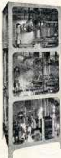
1000 Watt Master Oscillator Power Amplifier C. W. Radio Telephone Transmitter. Wavelength, 250 meters; height, 6 1/2 feet. REL inductances, variable and fixed condensers, R. F. choke coils, tube sockets, aluminum cast frames, etc.
