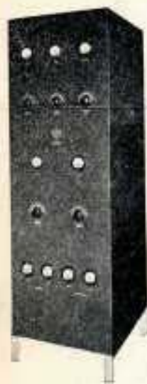
1000 Watt Master Oscillator Power Amplifier C. W. Radio Telephone Transmitter. Wavelength, 250 meters; height, 6 1/2 feet. REL inductances, variable and fixed condensers, R. F. choke coils, tube sockets, aluminum cast frames, etc.
