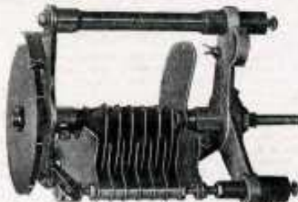
The above illustration shows the Cat. No. 187F condenser which is a combined, large capacity semi variable condenser shunted by a single plate small capacity variable condenser. The uses for this type are obvious. The idea is to spread narrow bands over the entire condenser tuning dial scale.
