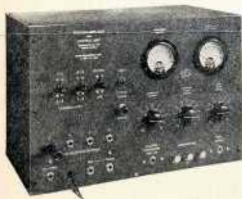
Broadest station line Amplifier and Control Unit. Completely controls the input to the transmitter. Wire telephone connections with each remote broadcast point. Automatic light signal devices.
