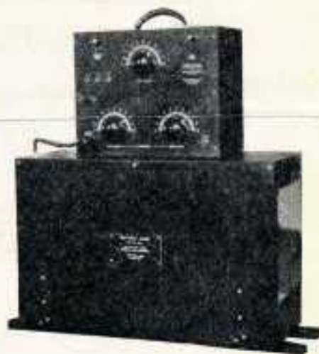
Portable Short Wave (combined) Transmitter and Receiver for Telephone and Telegraph operation. Employs two tubes for transmission and three tubes for reception. REL plug-in transmitting and receiving inductances, sockets, aluminum cast frames, etc. (Bottom compartment contains all batteries—actual set weighs only 22 pounds).
