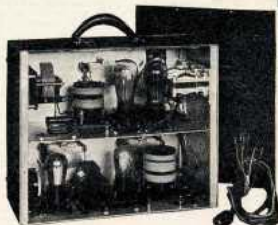
Rear View (Rear Panel Removed), Showing Plug-In Coils and Battery Cable
